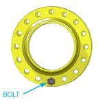
**3.** Repeat steps 1 and 2 at other points around the flange until all of the remaining bolt-holes are parallel and the rest of the bolts can be insterted.
