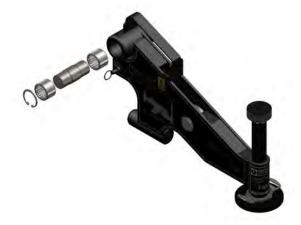
Remove the spirol retaining clips from the lower shaft and slide the shaft out from the main body.
