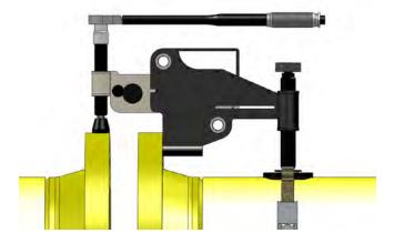
Loosen the wing retaining knob and extend the wing over to the opposite flange.
