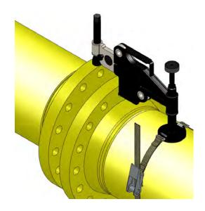
The torque wrench should be set at 19 Nm (14 ft·lb) then attached to the screw bolt.
