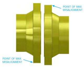
Guide the lift hook into the bolt hole at the point of maximum misalignment.
