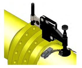
Tighten the screw bolt in a clockwise direction until the flanges come into alignment or the torque wrench "clicks".
